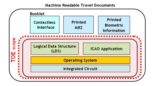
The TOE is defined to comprise the chip and the complete operating system and application. Note, the inlay holding the chip as well as the antenna and the booklet (holding the printed MRZ) are needed to represent a complete MRTD, nevertheless these parts are not inevitable for the secure operation of the TOE.
